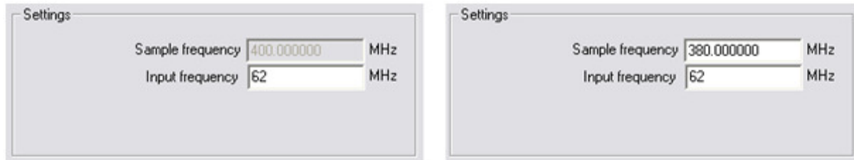
Figure 2. Sample frequency when running with internal clock (left) and external clock (right).
