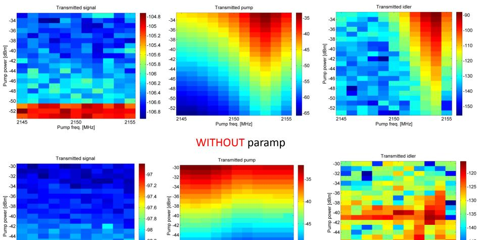
Input: circulator, combiner. Output: 2 circulators + HEMT. Assumed 53 and 50 dB pump attenuation with/without paramp
