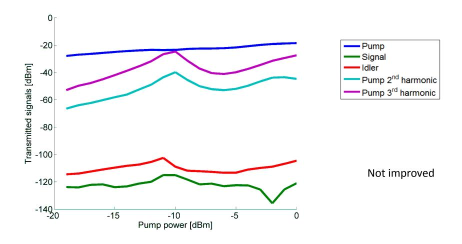
Wide scans (Pump = 20 dBm @ 2070 MHz), scanning signal frequency
