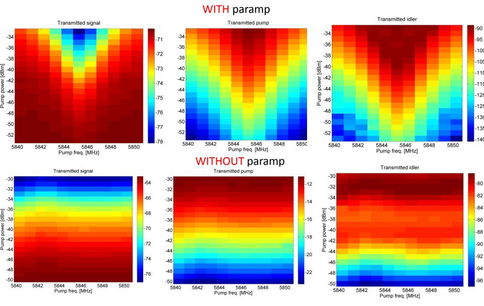
Input: circulator, combiner. Output: 2 circulators + HEMT. Assumed 53 and 50 dB pump attenuation with/without paramp
